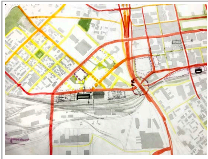
The macro-planning team analyzed the primary and secondary streets, and local streets of the zone. A primary street system challenge at Union Avenue and Water Street is marked by a circle.
