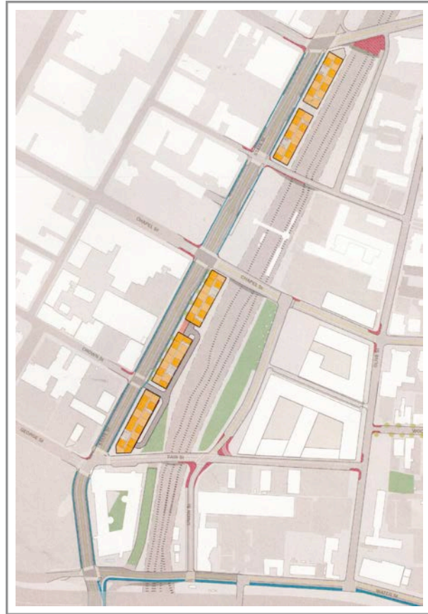
A plan developed by the City of New Haven for State Street between Water Street and Grand Avenue (Wooster Square TOD Study, 2016) narrows the roadbed to create parcels with sufficient depth along the East side of the street to allow new developments
